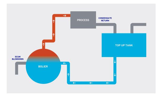
BWB have teamed up with Aquanet international, the world's only small footprint fully automated 24/7 boiler water monitoring and dosing company. Aquanet international provide complete water monitoring solutions adjusting dosing requirements dependant on boiler conditions and load. Contact them to discuss your requirements.
